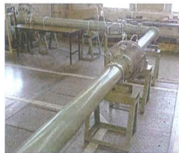
Flow test made by a flow test equipment according to the inspection regulations of CEN/TC 305/WG3/SG1 Study group (in the working group) for safety systems and devices for explosion protection of explosive gases in the CEN (European Standards Coordinating Committee).
